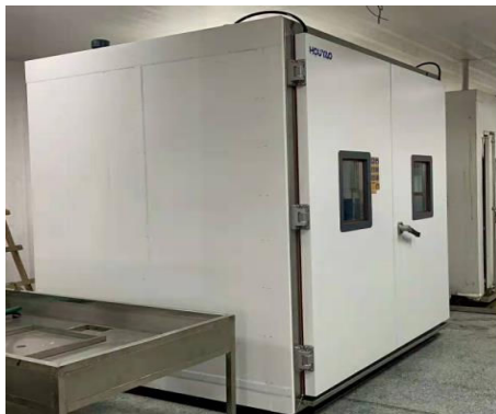
Instrument Name: Damp & Heat Testing Chambers Instrument manufacturer: Shanghai Houyao Model: HY-BRS-DH-9
